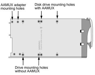
Figure 8. SATA drive mounted in a drive carrier with the required AAMUX adapter
